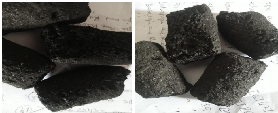
Fig. 1. Bio- briquette produced from groundnut shell.
